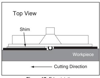
**Figure 17.** Edge jointing (guard removed for clarity).
